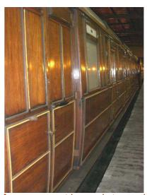
Meanwhile at the 'Stourport end', which will remain in its original "Pigeon Van" form, great strides are being made to clean, de-bug, repair and recycle enough of the original planking to clad the interior. About half the planks have been completed and fitted with enough for a third section. The fourth and final section includes the space in front of the guard's compartment, for which we *may* need to buy some new planking.
