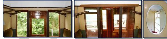
The lino has been laid at the passenger end, and the luggage racks are also in progress. Other completed items are the newly-made underseat grills to protect the heater elements from inquisitive young fingers. The WC has gained a mirror – not a genuine LNER item, which would be too tempting to thieves, but it looks the part – and the WC seat has its glorious varnished finish.
