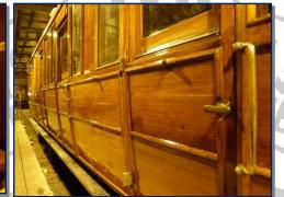
Our project vehicle is now receiving some of its finishing touches in Kidderminster's Carriage Shed. It has had four more coats of varnish, making at least ten coats (some areas more). The body is now ready to be lined out, numbered and lettered prior to final varnishing. Its overhauled bogies can soon be fitted, along with the corridor bellows. The mechanical and electrical overhauls will be done when a
