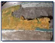
We have now started the big task of replacing the life-expired roof canvas on Tourist Third Open 43600. This is being done as a volunteer-led project in Kidderminster's Carriage Shed – which has its own unique microclimate especially in freezing weather. The first stage of stripping the old canvas has proved rather challenging in the winter cold.
