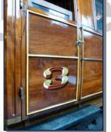
This major overhaul is at last coming together at Kidderminster. Bodywork repairs are done; teak panels are back on the framing; the new more robust seating is being installed; and varnishing has begun. The vehicle is needed back in the teak set so as to provide an acceptable attractive seating area for our passengers who use wheelchairs.
