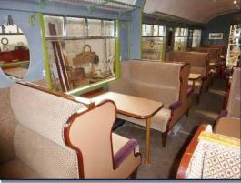
Steady progress here. The body overhaul is largely done. The roof timbers are secure again with nearly 1000 new bolts holding them firmly into the steel frame hoops; and the new roof canvas has its traditional white finish. The new tables, the redesigned & reupholstered seats and other fixtures
