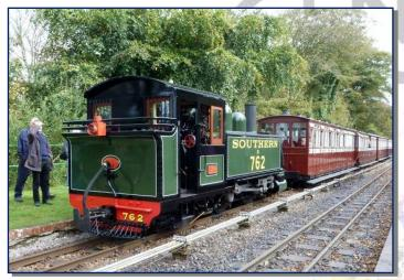
The editor has nodded off again, but that allows a mention of this historic milestone with completion of a new-build engine replicating the L&B's original 'Baldwin' loco LYN. The engine was built by Alan Keef Engineering near Ross-on-Wye. It incorporates improved design features such as roller bearings and a higher boiler pressure compared with the long-scrapped original.
