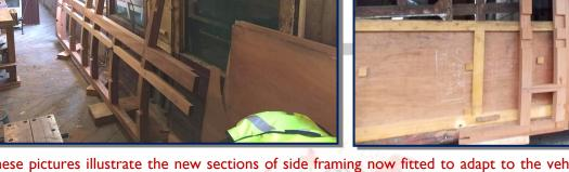
These pictures illustrate the new sections of side framing now fitted to adapt to the vehicle's new function. They show what will be the buffet bar wall, along with the end-door on the bar side and a trial fit of a window toplight. Further fuller information about this important project is at: <a href="http://www.lnersvrcoachfund.org.uk/gwr5043.html">http://www.lnersvrcoachfund.org.uk/gwr5043.html</a>
