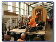
We've just heard that the LNER Coach Association have successfully moved the body of their East Coast Joint Stock clerestory dining car No.189, built in 1894. It had been on a temporary underframe, but it now rests on its permanent frame, which has been modified to suit the shorter body length. The body has already had substantial repairs, and the way is now open for the serious restoration of its once
